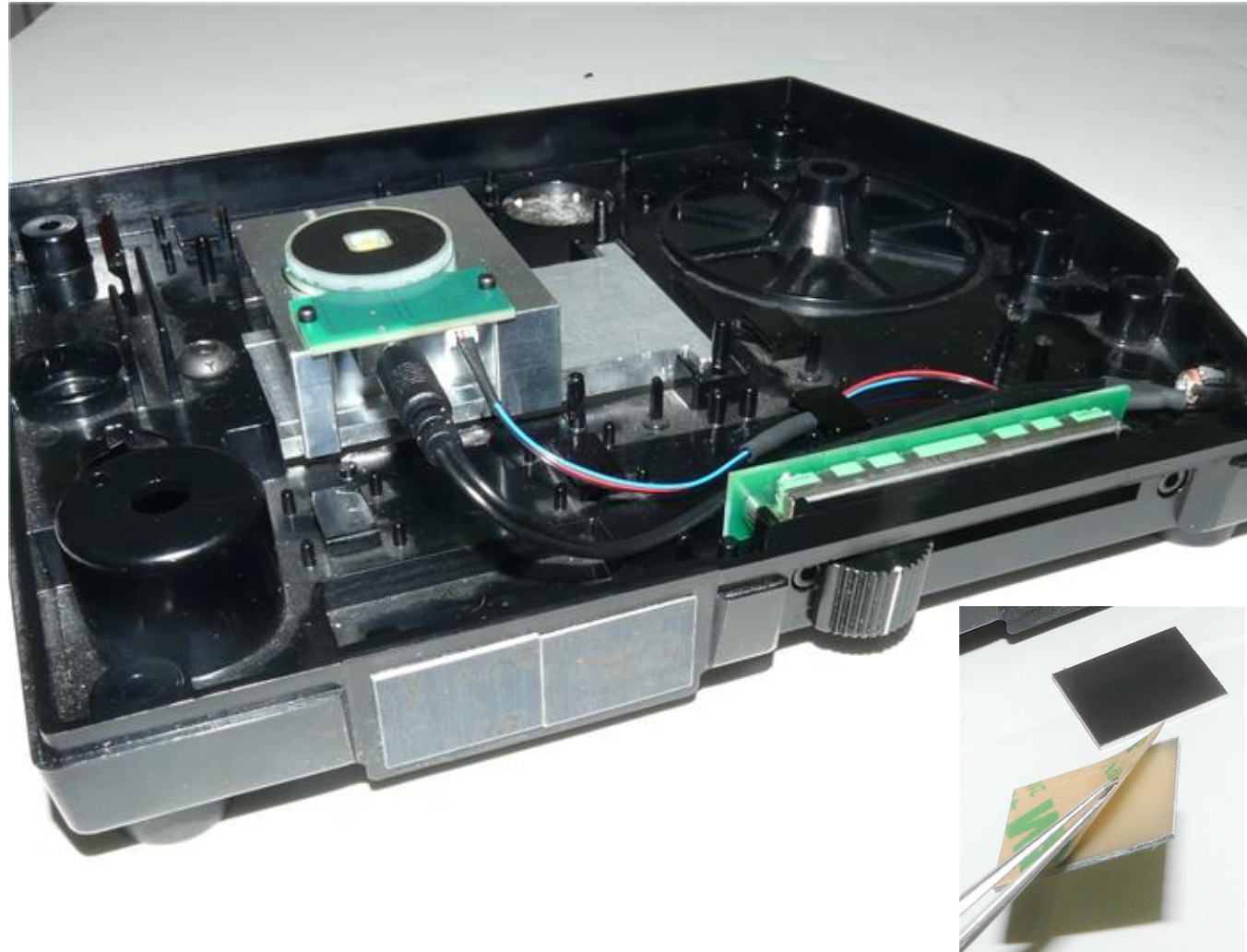
(1) Remove the release film from the back of the blank off plates as shown above in the inset photo. Then attach them as shown in the main photo to cover the hole where the switch was.
