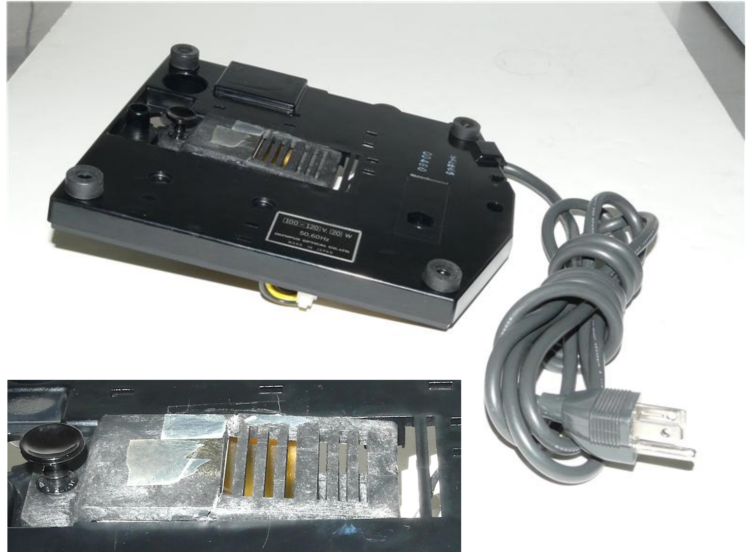
(2) Bottom view of microscope base. Note severe heat damaged plastic "trap door" which has cracked and broken. This will be replaced with an aluminum part.
